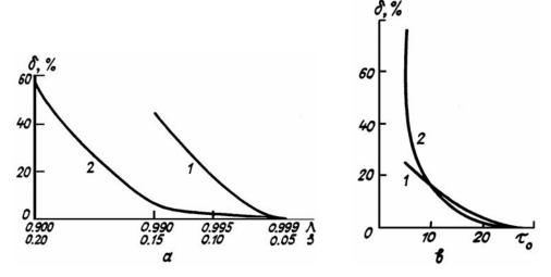
FIG. 1. Relative errors in determining  $\tau_0$  and s from the formulas (21) and (22) ( $\delta \tau$  is indicated by curve 1 and  $\delta s$  is indicated by curve 2; g = 0.85): a) as a function of  $\Lambda$  for  $\tau_0 = 25$  and b) as a function of  $\tau_0$  for  $\Lambda = 0.999$ .
