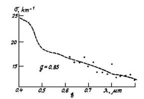
FIG. 2. Spectral dependences: a) hemispherical fluxes of diffuse solar radiation emanating from the cloud layer derived from the data of Ref. 1 (curve 1 indicates  $F^{\uparrow}$ ,  $2 - F^{\downarrow}$ , and 3 - A; b) volume light scattering coefficient; and, c) volume coefficient of real light absorption.
