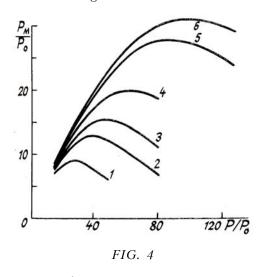
Figure 4 shows power optimization curves of the same beam with the use of a modal corrector: 1) without correction; 2) tilt correction; 3) tilt and defocusing correction; 4) tilt, defocusing, and astigmatism corrections; 5) corrections of the first seven aberrations; and, 6) correction of eight aberrations.
