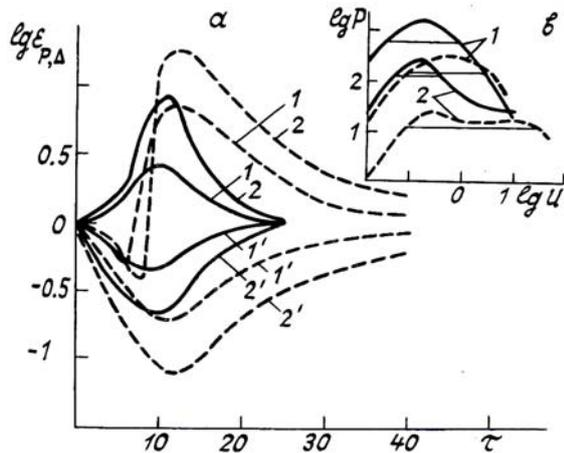
FIG. 1. Ratios of the amplitudes  $\varepsilon_p$  (1' and 2') and durations  $\varepsilon_\Delta$  (1 and 2) of the pulses when the detector is located at the distances  $\tau_0 = 33.33$  (1 and 1') and 166.7 (2 and 2') from the layer and at the layer boundary for the receiving angles  $10^\circ$  (solid lines) and  $90^\circ$  (dashed lines).
