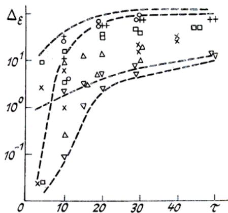
FIG. 4. Energetical pulse duration  $\Delta_\epsilon$  in units of  $10^{-6}$  sec as a function of the optical thickness  $\tau$  of the layer for different types of cloudiness.
