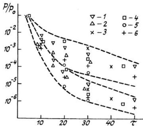
FIG. 2. Relative amplitude  $P_m/P_0$  of the transmitted pulses ( $P_0$  is the amplitude in the absence of cloudiness) as a function of cloud optical thickness for different types of cloudiness: St (1), As (2), St + As (3), St + Ci (4), As + Ci (5), St + As + Ci (6).
