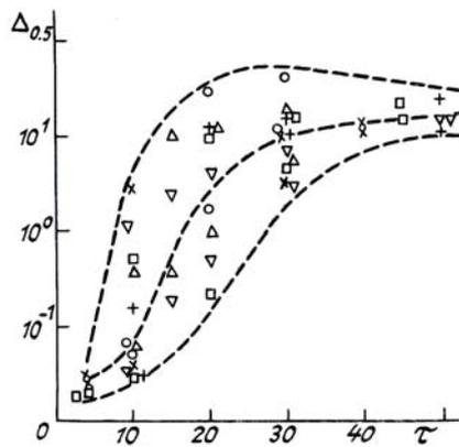
FIG. 3. Pulse duration  $\Delta_{0.5}$  in units of  $10^{-6}$  sec as a function of the layer optical thickness  $\tau$  for different types of cloudiness.
