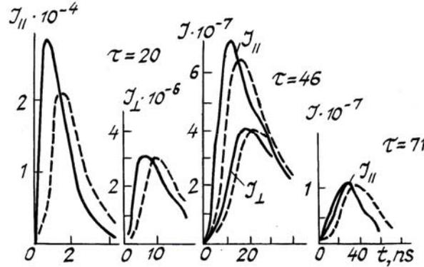
FIG. 3. Comparison of experimentally recorded pulses with those calculated by the SADA formulas
