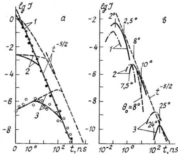
FIG. 4. Pulse shapes obtained by numerical calculations (a) and by SADA (b) for different detector angular displacements from the beam axis: 1 –  $\alpha = 0.5^\circ$ ; 2 –  $\alpha = 2^\circ$ ; 3 –  $\alpha = 10^\circ$ .
