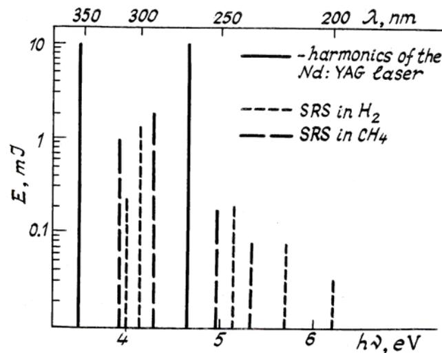
FIG. 2. The spectrum of the laser source.
