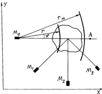
FIG. 1. Coordinate system and location of the acoustic detectors  $M_0 - M_3$ .
