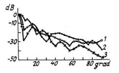
FIG. 2. Directional pattern of a selective acoustic antenna: 1) directional pattern of the horn; 2) directional pattern of an antenna with phase reversal in the even Fresnel zones; 3) same, but with phase reversal in the odd Fresnel zones.
