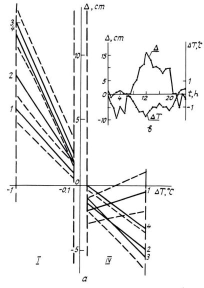
FIG. 1. Refraction distortions: experimental vs computed regression lines (based on formula (2), for a distance of 500 m).
