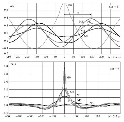
Fig. 3. Coefficients of time correlation of acoustic wave. M0 is the coefficient of autocorrelation of the first microphone, M1... M4 are the coefficients of cross-correlation between the microphone M0 and microphones M1, M2, M3, M4;  $\phi$  is the phase shift.
