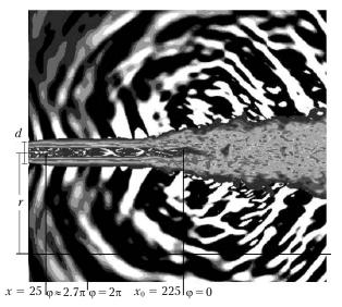
**Fig. 5.** The results of numerical simulation of acoustic field<sup>8</sup> as compared with data on the phase shift in the configuration of Fig. 1a.
