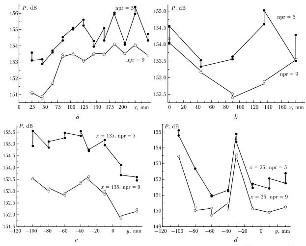
**Fig. 6.** The level of acoustic oscillations at npr = 5 and 9 with configurations: along the axis (*a*), in a circle (*b*), in the transversal section at x = 135 mm (*c*) and x = 25 mm (*d*).
