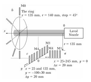
Fig. 1. Configurations of microphones in the Eifel chamber.
