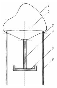
Fig. 1. The device for collecting dry aerosols.
