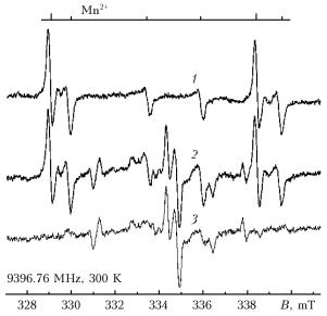
Fig. 3. EPR spectrum of organic radicals on the CaCO<sub>3</sub> surface: standard sample (1); exhibited sample (2); a focused signal of organic radicals in the exhibited sample (3). B, mT (polarizing magnetic field in millitesla).
