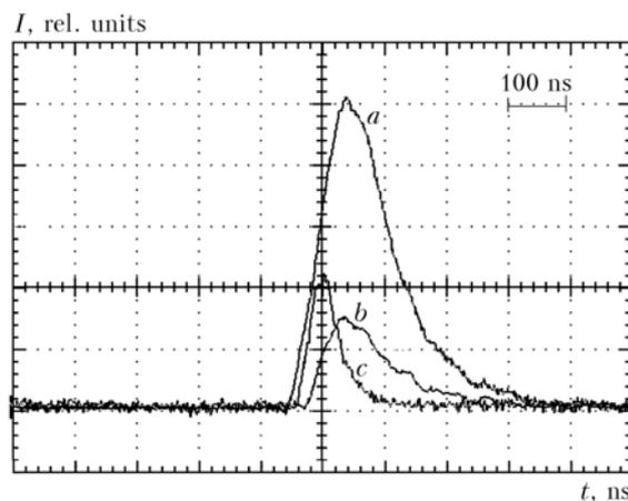
Fig. 2. The shape of strontium-vapor laser generation pulse: *a* is the total pulse; *b* is a 3  $\mu\text{m}$  pulse, *c* is a 1  $\mu\text{m}$  pulse.
