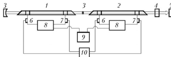
**Fig. 1.** A master oscillator-power amplifier system: gas-discharge tube of the oscillator (1); gas-discharge tube of the amplifier (2); unstable telescopic resonator (3); filter bank (4); power meter (5); current bypass (6); voltage divider (7); power source (8); master oscillator (9); oscillograph (10).
