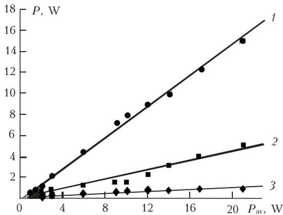
**Fig. 4.** Average radiation power distribution over spectral lines in the master oscillator-power amplifier system: generation power at 6.456  $\mu\text{m}$  line (1); total generation power at 3 (2) and at 1  $\mu\text{m}$  (3).
