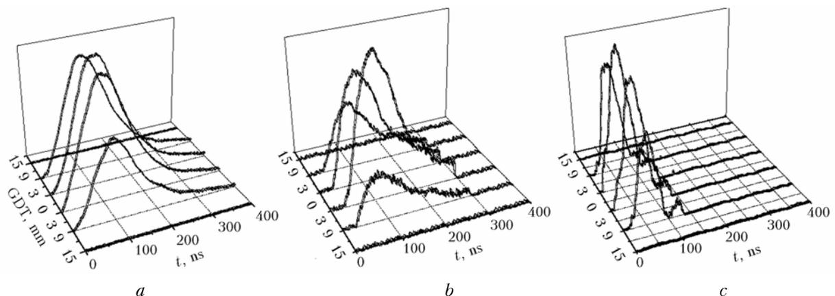
Fig. 3. Variability of generation pulse shape depending on the diameter of the discharge channel: total generation pulse (*a*); 3- $\mu\text{m}$  pulse (*b*), 1- $\mu\text{m}$  pulse (*c*).
