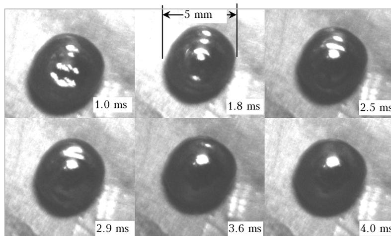
**Fig. 2.** Dynamics of relaxation of the liquid gallium drop surface. Exposure time of each frame is 1 μs, the interframe times are: 1; 1.8; 2.5; 2.9; 3.6; and 4 ms after the irradiation. The beam incidence is normal to the picture. The ablation region is in the drop center.
