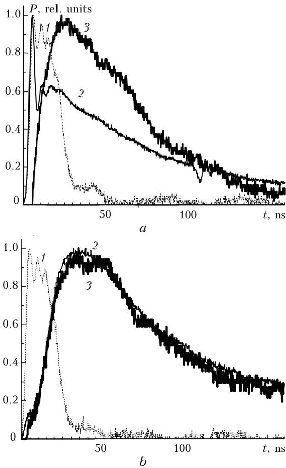
**Fig. 1.** The oscillograms of laser pulse (1) and plasma luminosity pulses on the surface of heavy (a) and liquid (b) Wood alloy at 200–600 (2) and 340–600 nm (3) wavelengths in the neon atmosphere at a pressure of 370 Torr.
