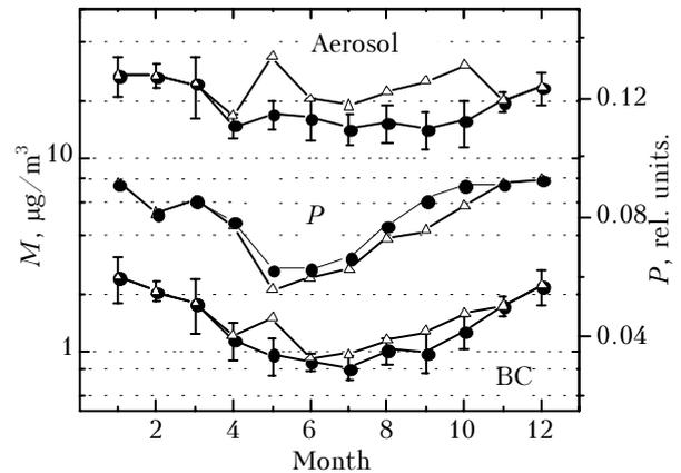
**Fig. 3.** Annual behavior of concentrations of  $M_a$ ,  $M_{BC}$ , and  $P$  (1997–2006): taking into account fires (open triangles) and background aerosol (closed circles).
