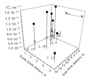
**Fig. 6.** Structural parameter of the refraction index  $C_n^2$  inside the spectrograph pavilion. The black circles correspond to measurements at the lower level (p. 1-7) and the white one – at the upper level (p. 8-12): input window (1), diffraction grating (2); output slits (3); diagonal mirror (5 and 10); chamber mirrors (6, 7, 11, and 12), and over the adjustment table (8).
