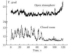
Fig. 8. Two-minute realizations of the random temperature T in a closed room and in free atmosphere.
