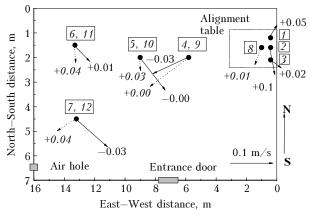
**Fig. 2.** Spectrograph pavilion. Scheme of measurements in the pavilion (overhead view) and wind map. Numbers inside the rectangles are the numbers of measurement points; numbers near the arrays' ends with the signs \*+ or \*- are the values of vertical wind (m/s). Solid arrows and non-italic numbers correspond to the velocity at the floor of pavilion (1–7), dashed arrows and italic numbers – at the top of pavilion. Velocity scale is shown in the right bottom angle.
