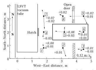
**Fig. 4.** Adaptive table. Measurement scheme (side view) and wind map. Numbers inside the rectangles are the numbers of measurement points; numbers near the measurement points with the signs  $\ll \gg$  or  $\ll \gg$  correspond to the values of vertical wind (m/s). Solid arrows and non-italic numbers correspond to the velocity at the floor of the room (1-9), dashed arrows with italic numbers – at the top of the room (1, 3, 5–7, 9). Horizontal velocity scale is shown in the right bottom angle.
