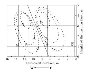
Fig. 7. Air motion inside the pavilion in a vertical plane through points 2 and 4-6 (their positions are designated by italic numbers). Ellipses show the trajectories of averaged motions, slant solid line – the projection of smoothed average temperature gradient.
