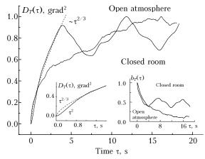
**Fig. 9.** Normalized structure  $D_T(\tau)$  and correlation  $b_T(\tau)$  (right bottom subfigure) functions in a closed room and in open atmosphere (the initial segment of  $D_T(\tau)$  is shown at the bottom left).
