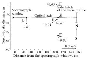
Fig. 5. Working place of spectrograph operator. Measurement scheme (overhead view) and wind map. Numbers in the rectangles are the numbers of measurement points. Arrows are the horizontal wind velocities (the scale is in the right bottom angle). Numbers near the arrows' ends with the signs \*+ or \*- correspond to the vertical wind values, m/s.
