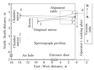
**Fig. 1.** Scheme of the LSVT astronomic spectrograph (overhead view).
