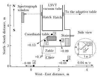
**Fig. 3.** Coordinate table. Scheme of measurements around the table (overhead view) and wind map. The subfigure in the right bottom angle presents the side (west) view. Numbers inside the rectangles are the numbers of measurement points. Solid arrows correspond to the horizontal velocity (the scale is shown in the right bottom angle). Numbers near the arrows' ends with the signs  $\ll \ast$  or  $\ll \ast$  correspond to the values of vertical wind, m/s.
