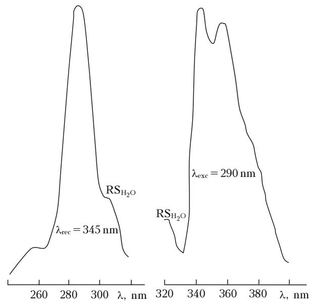
**Fig. 2.** Spectra of excitation and UV fluorescence in part *a* of the centrifuged seawater sample collected from a depth of 20 m ( $RS_{H_2O}$  is the Raman scattering of water).
