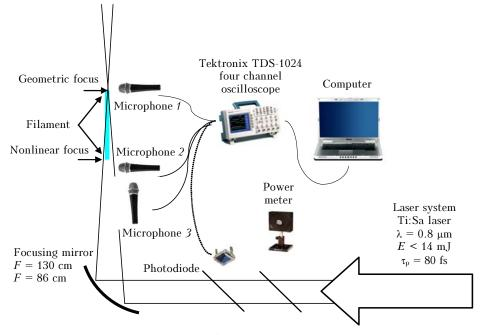
Fig. 1. Block diagram of the experiment.
