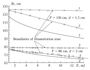
**Fig. 4.** Positions of the beginning (2, 4) and end (1, 3) of the filamentation zone for two focusing mirrors as functions of the input beam energy; (5, 6) theoretical dependences.
