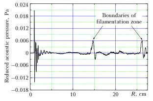
**Fig. 2.** Time scan of the acoustic signal generated by a laser beam and measured in the longitudinal direction. The acoustic pressure is reduced to a distance of 1 m:  $P_{\text{ac.red}} = P_{\text{ac.m}}R$ .
