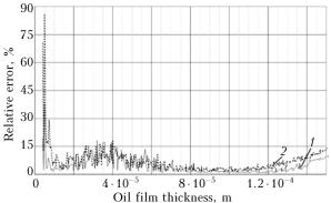
**Fig. 3.** The dependence of mean error of the determination of the oil film thickness on the real value of the thickness in a series of 30 measurements.
