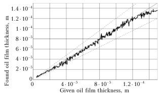
**Fig. 2.** The dependence of the found oil film thickness value on the real thickness value in the case of averaging the results over a series of 30 measurements.
