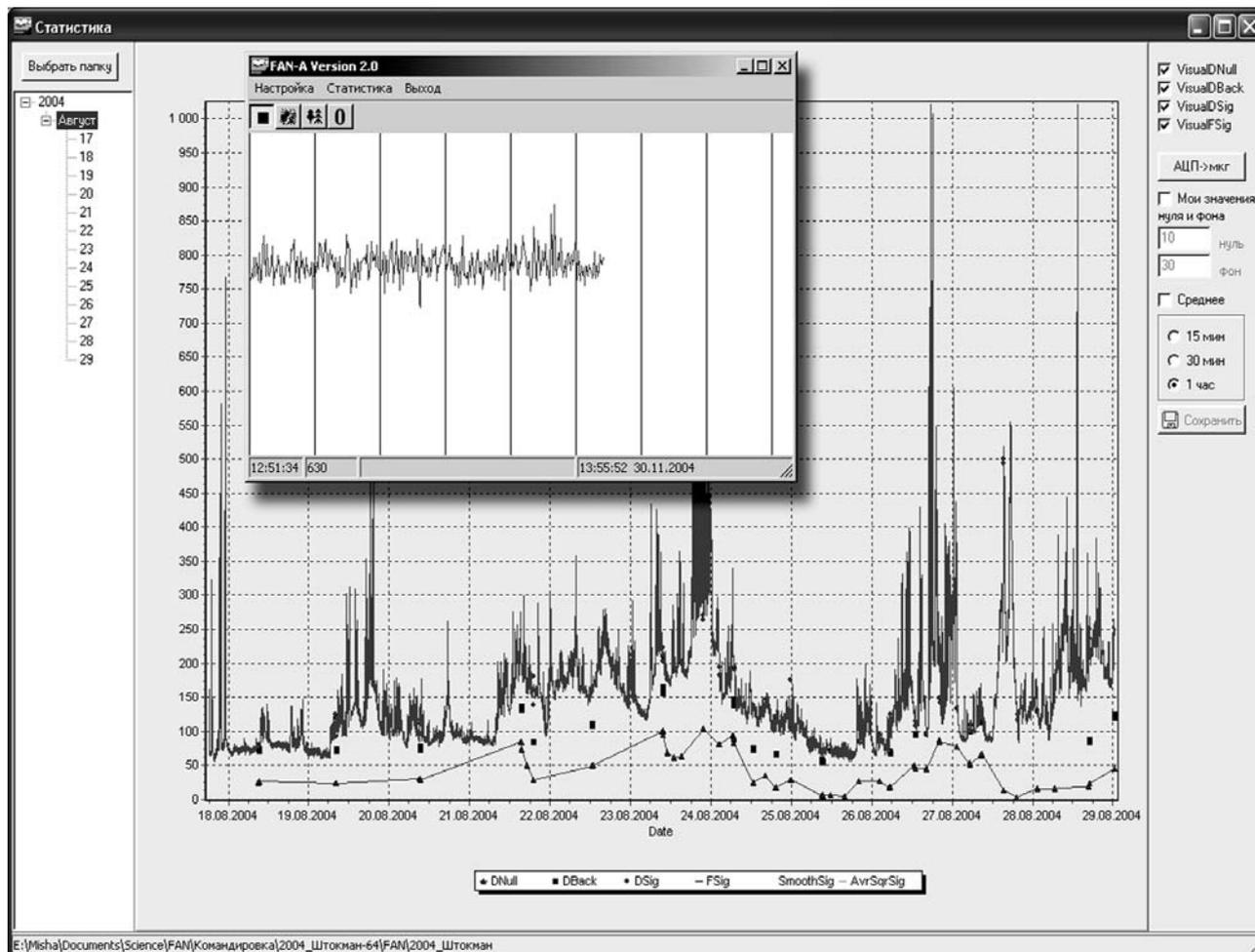
Fig. 4. Graphic interface of the program controlling the nephelometer controller. The controlling window with second-to-second imaging of the signal is at the top to the left (the interval between vertical lines is 1 minute). The whole signal with a minute resolution is at the bottom.
