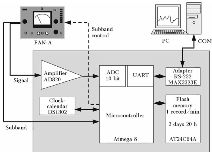
Рис. 2. Schematic view of the nephelometer microcontroller board.
