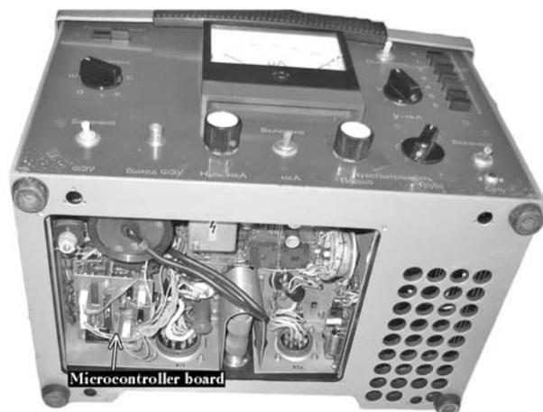
Fig. 3. FAN-A nephelometer. The microcontroller board is inside its casing.
