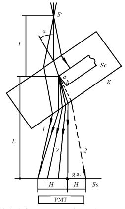
Fig. 1. Optical arrangement of experiments on light diffraction by a screen placed in the air or in a liquid.
