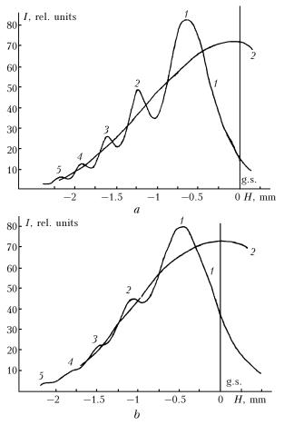
**Fig. 2.** IKS3-plate diffraction pattern when the plate is in air (*a*) and in dimethyl phthalate solution in benzyl alcohol at  $n_{\rm rel} = 1.0054$  (*b*).
