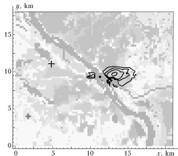
**Fig. 1.** Calculation area and concentration isolines. The source is marked by the cross.
