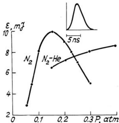
Fig. 4. The radiation energy as a function of the  $\text{N}_2$  and He content. The inset shows the radiation pulse of a  $\text{N}_2$  laser.
