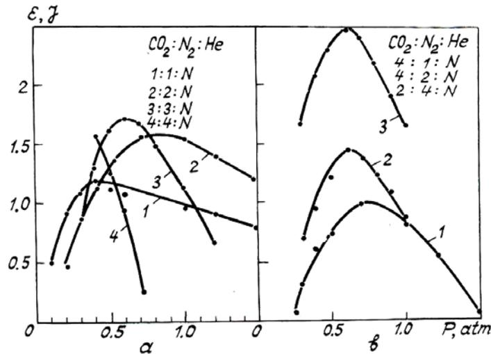
Fig. 3. The optimal dependences of the radiation energy on the content of  $\text{CO}_2$ ,  $\text{N}_2$  (a), and  $\text{N}_2$  (b) and the total working pressure of the mixture with  $U_0 = 30$  kV.
