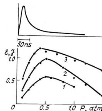
Fig. 1. The energy of radiation for the gas mixture CO<sub>2</sub>:N<sub>2</sub>:He = 1:1:N as a function of the helium content and the magnitude of the charging voltage: 20 kV (1), 25 kV (2), and 30 kV (3). The graph at the top shows the radiation pulse in a mixture with no helium CO<sub>2</sub>:N<sub>2</sub> = 4:1.
