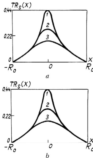
FIG. 1. The response of a membrane mirror to the action of an actuator at the center ( $r_s = 0$ ): a)  $D_0 = 0$ : 1 -  $r_a = 0.1 R_0$ , 2 -  $r_a = 0.3 R_0$ , 3 -  $r_a = 0.5 R_0$ , b)  $D_0 \neq 0, r_a = 0$ : 1 -  $\omega = 2$ , 2 -  $\omega = 20$ .
