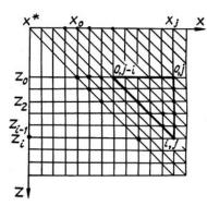
FIG. 1. A discrete scheme for two-beam tomographic sounding of the atmosphere.
