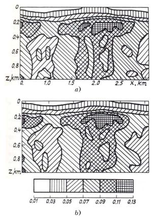
FIG. 2. The reconstruction of the two-dimensional spatial distribution of the backscattering coefficient  $\beta(x, z)$  in a numerical experiment: a) model distribution  $\beta_0(x, z)$ ; b) result of the solution of the inverse problem with a 10%-error in the lidar signals.
