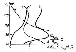
FIG. 1. Theoretical vertical profiles of the reconstruction errors: curve  $1 - \sigma_T(z)$  with known composition (two-channel measuring system); curve  $2 - \sigma_T(z)$  with unknown composition (three-channel measuring system); curve  $3 - \sigma_A/\Lambda_{10}$  with unknown composition; curve  $4 - \sigma_{CO_2}/q_{CO_2}$ .
