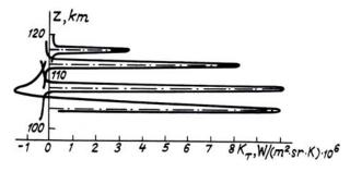
FIG. 2. The weighting function of the three-channel method for reconstructing the temperature,  $K_{T,1,2,3}(h, z')$ . The dot-dashed lines mark the tangential sounding heights.
