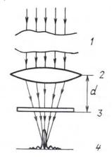
FIG. 1. Schematic of Image Correction: 1) distorting medium; 2) lens; 3) phase corrector; 4) image plane.
