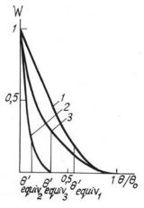
FIG. 4. Optical transfer function: 1) ideal OTF; 2) OTF in a turbulent medium; 3) OTF with correction applied.
