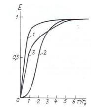
FIG. 3. Energy distribution over the blur circle: 1) no distortions; 2) phase fluctuations with  $D_s(\emptyset) = 5.26 \text{ rad}^2$ ; 3) phase correction by adaptive mirror;  $r_0$  is the Airy radius.
