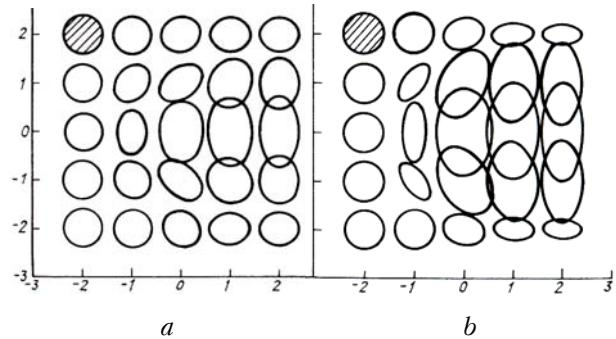
FIG. 3. Transformations of the coherence ellipse over the Gaussian beam cross-section calculated in the geometric — optics approximation at the distances  $z = 1$  (a) and  $z = 1.5$  (b). The cross-hatched part of the figure shows the undisturbed normalized coherence ellipse in the starting plane.
