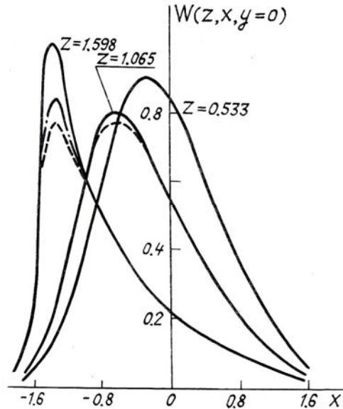
FIG. 4. Comparison of the calculations of the self-action of partially coherent radiation (solid curves) and coherent radiation: the results of Ref. 10 ( $E_r = 123$ ) and Ref. 11 ( $E_r = 246$ , dot-dashed curves.).
