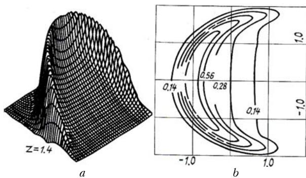
FIG. 1. The aberrational structure of a Gaussian beam obtained in the geometric optics approximation (a) and isopleths for the intensity of the same beam (b).
