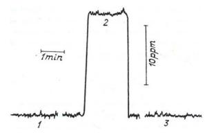
FIG. 4. Readings of the HHC sum analyzer. Curve 1 was obtained when only methane was present in the hydrocarbon-air mixture ( $C_m = 5 \times 10^2$  ppm). Curve 2 was obtained for a mixture of methane and propane with air ( $C_m = 2.2 \times 10^2$  ppm,  $C_{pr} = 1.7 \times 10^1$  ppm). Curve 3 is the analyzer baseline.
