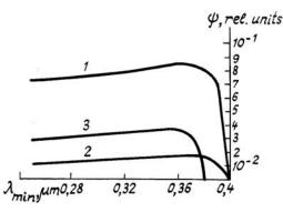
FIG. 1. The SNR versus the short-wavelength limit of the sensitivity zone: 1)  $\lambda_{max} = 0.4 \ \mu m$  and the underlying surface is snow covered; 2)  $\lambda_{max} = 0.4 \ \mu m$  and the underlying surface is covered with vegetation; 3)  $\lambda_{max} = 0.38 \ \mu m$  and the underlying surface is snow covered.
