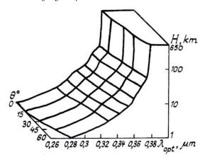
FIG. 2. Altitude and angular dependence of the optimal short-wavelength boundary for a meteorological visibility range of 50 km and a snow-covered underlying surface.
