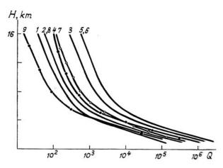
FIG. 2. Profiles of SNR Q for ground-based lidar. E = 0.065 J(1), 0.1(2, 8, 9), 0.5(3, 4, 7),and 1(5, 6); for curves 4 and 9  $C_{n0}^2 = 10^{-12} m^{-2/3}$  and for the other curves  $10^{-14} m^{-2/3}$ ; for curve 8  $\xi = 200$  and for the other curves  $\xi = 100$ ; for curve 7  $\Delta R = 300$  m and for the other curves 750 m.
