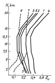
FIG. 5. The relative error  $\delta_v$  versus the altitude H for a space-lidar. For curves 6 and 7 v(H) = 30 m/sec; for the other curves see the caption to Fig. 4.
