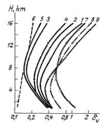
FIG. 3. The relative error  $\delta_v$  versus the altitude H for a ground-based lidar. For curve  $\delta_v(H) = 30$  m/sec; for the other curves see caption to Fig. 2.
