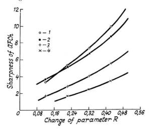
FIG. 3. Comparison of the selective properties of an anisotropic resonator and resonators with Fabri-Pero and Fox-Smith interferometers. Key: 1) Sharpness of AFC 2) Change in the parameter R.
