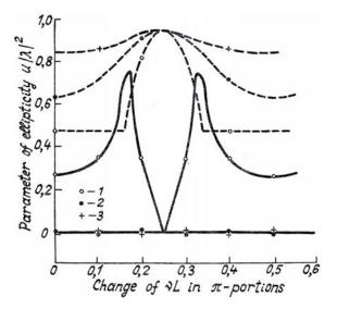
FIG. 4. The ellypticity and the values of the AFC for different values of  $\beta$  and P: 1)  $\beta = 0$ ; P > 0; 2) P = 0; 3)  $\beta = \pi/4$ , P > 1. Key: 1) Ellipticity and  $|\Lambda|^2$
