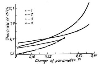
FIG. 2. The sharpness of the AFC of the optical system under study as a function of the properties of the polarizer: curves 1 and 3 are for a quarter-wave LPP and curves 2 and 4 are for a "thin" LPP. Key: 1) Sharpness of AFC 2) Change in the parameter P.
