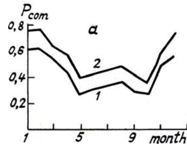
FIG. 3. Annual behaviour of communication probability in Tompo. 1 - 5 dB attenuation, 2 - 50 dB attenuation.
