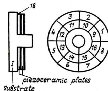
FIG. 2. Adaptive mirror design substrate; piezoelectric-ceramic plates
