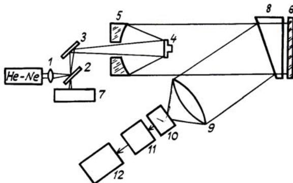
FIG. 1. Optical scheme: 1 – microscope objective; 2 – split mirror; 3 – tilt corrector; 4 – adaptive mirror; 5 – spherical mirror; 6 – reflector; 7 – wavefront sensor; 8 – wedge-shape splitter; 9 – objective 10 – microscope; 11 – TV-camera; 12 – buffer memory.
