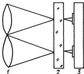
FIG. 3. Wavefront Hartmann sensor 1 – lens raster; 2 – glass-fiber plate; 3 – photodetector array
