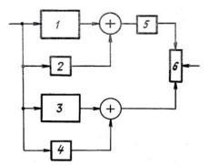
FIG. 1. Block diagram of the electrical model of the atmosphere. Here 1 and 3 are low-pass filters modeling the best and the worst observation conditions; 2, 4, and 5 are the delay lines for 1, 2, and 3; 6 is potentiometer.
