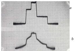
FIG. 3. Oscillograms of the electrical test-signal for a TV system; (a) is the case with no aperture distortions; (b) represents the case involving distortions introduced by the opto-electronic channel of the system and by the scattering properties of the atmosphere.
