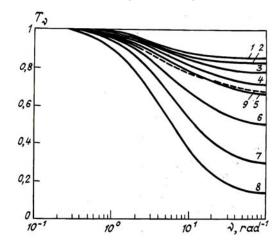
FIG. 2. Approximation of calculated FCC of the atmosphere by frequency response of the electric model. Curves 1 to 8 correspond to  $V_{\rm M}$  from 250 km to 3 km. The height of the observation is platform H = 5 km, the wavelength  $\lambda = 0.35$  µm. Curve 9 presents an example of the calculated FCC of the atmosphere.
