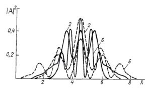
FIG. 1. Profiles of the intensity of the optical radiation propagating through a linear medium for Gaussian-shape pulses at the time t = 1.19 and cross-sections z = 0.1 (solid curves), z = 0.2 (dashed curves). The values of the parameter m are shown near the curves;  $x_0 = 4.5$ .
