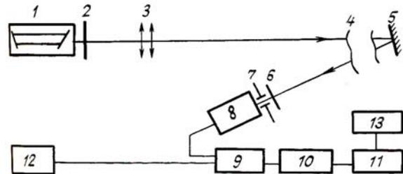
FIG. 2. Experimental setup: 1) laser, 2) neutral filter, 3) telescope, 4) atmosphere, 5) mirror, 6) interferent filter, 7) diaphragm, 8) photomultiplier, 9) former, 10) counter, 11) interface, 12) frequency meter, and 13) computer.
