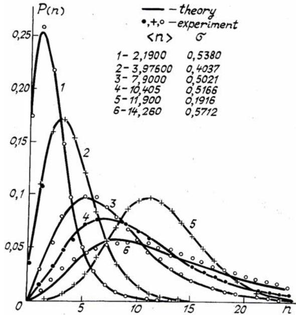
FIG. 3. PPD curves for laser radiation along an atmospheric path with length  $2l = 100$  m at different radiation levels and degree of turbulence: solid curves theory, points-experiment: theory; points experiment:  $\langle n \rangle = 2.19$  and  $\sigma = 0.538$  (1), 3.976 and 0.4037 (2), 7.9 and 0.5021 (3), 10.405 and 0.5166 (4), 11.9 and 0.1916 (5), and 14.26 and 0.5712 (6), respectively.
