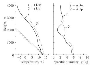
Fig. 1. Vertical distribution of air temperature and specific humidity during one of summer airborne investigations in Norilsk. Here and further the measurement designations: Up - during take-off, Dw - at landing.
