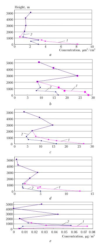
**Fig. 5.** Vertical distribution of the volume aerosol concentration (*a*); vertical distribution of identified aerosol (*b*); vertical distribution of ions (*c*) and  $SO_4^{2-}$  ions (*d*); vertical distribution of lead containing compounds (*e*): all samples (curve 1), out of plume (2).
