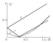
**Fig. 2.** Dependences of the interferometer sensitivity factors at the fixed values of f = 220 mm,  $l_1 = 220$  mm,  $l_2 = 300$  mm:  $G_1(1)$ ,  $G_2(2)$ ,  $G_3(3)$ .
