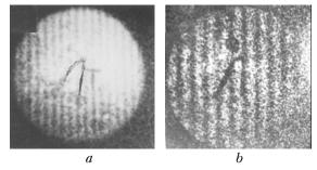
**Fig. 6.** Interference patterns, localized in the plane of the diffuser image formation and characterizing its cross motion: for the illumination of the diffuser with radiation of a diverging spherical wave (a); for the case of illumination with a converging spherical wave (b).
