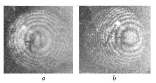
**Fig. 8.** Interference patterns, localized in the plane of the diffuser image formation, characterizing its longitudinal motion and recorded while performing spatial filtering of the diffraction field in the hologram plane: the filtering on the optical axis (a); for that outside the optical axis (b).
