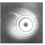
**Fig. 9.** Interference pattern, localized in the plane of the Fourier hologram and characterizing the cross and longitudinal motions of a flat diffuser.
