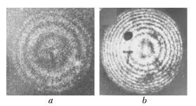
**Fig. 7.** Interference patterns, localized in the plane of the diffuser image formation and characterizing its longitudinal motion: for the distance  $l_2 = 300 \text{ mm}(a)$ ; for  $l_2 = 180 \text{ mm}(b)$ .
