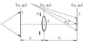
**Fig. 1.** Diagram of the double-exposure recording of the quasi-Fourier hologram: t is the matte screen; 2 is the photographic plate; L is the positive lens; p is the aperture diaphragm.
