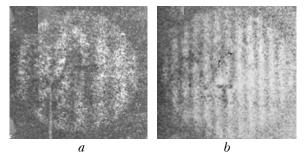
Fig. 4. Interference patterns, localized in the plane of the diffuser image formation and characterizing its cross motion: the illumination of the diffuser with the radiation of a diverging spherical wave (a); of a converging spherical wave (b).
