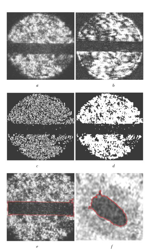
Fig. 5. Examples of the instrumental and numerical processing of holographic images, including the detection of boundaries: (a) initial image; (b) result of the instrumental processing using the optical set up shown in Fig. 2b; (c) numerical processing by the gradient filter; (d) numerical processing by the Sobel's filter; (e, f) results of operation of the algorithm, detecting the boundaries.
