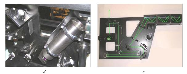
Fig. 1. General view of the simulator (a, b) and its optical arrangement (c); module for formation of the object beam: (d) as a part of the simulator; (e) separately from the simulator; the light line shows the beam path; (c) beam-turning mirror 1, beam splitter 2, collimators (Galilean telescopic system) 3 and 4, glass cell modeling the studied volume 5, optical system of image transfer (Keplerian telescopic system) 6, mirror system 7; photoplate 8.
