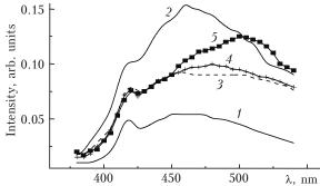
**Fig. 2.** Fluorescence spectrum of HSs in water-alkaline solutions  $C_{\rm HS} = 0.0098$  g/1 and  $C_{\rm NaOH} = 0.0019$  m/l;  $\lambda_{\rm pump} = 365$  nm; HS from the Merck peat (1), chernozem (2), sod-podzol (3), brown coal (4), and podzol (5).
