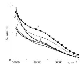
Fig. 1. Absorption spectrum of HS in the water-alkaline solution at  $C_{\rm HS} = 0.0098$  g/l,  $C_{\rm NaOH} = 0.0019$  m/l: HS from the Merck peat (1), chernozem (2), sod-podzol (3), brown coal (4), and podzol (5).
