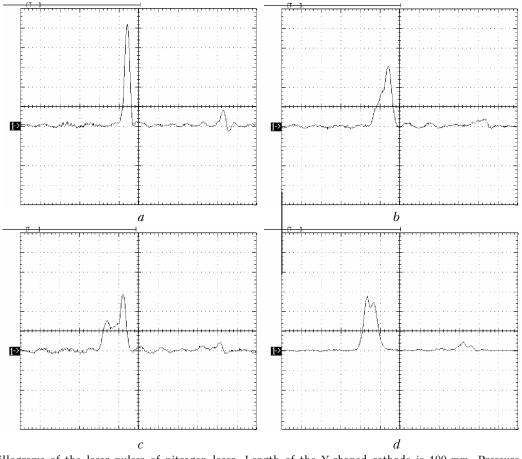
**Fig. 6.** Oscillograms of the laser pulses of nitrogen laser. Length of the Y-shaped cathode is 100 mm. Pressure in the laser cell: 6.6 (*a*); 11.6 (*b*); 18 (*c*); 49.5 Torr (*d*). The vertical scale: 32 V/div (*a* and *b*) 16 V/div (*c*); 64 V/div (*d*); (*a*)-(*c*) a negative lens was used for signal attenuation; *d* the lens was not used because of the low sensitivity of the recorder. The horizontal scale is 10 ns/div.
