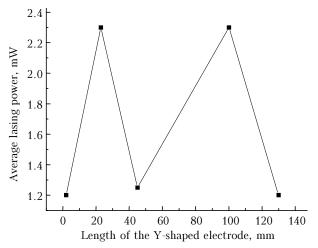
**Fig. 4.** Dependence of the average radiation power of the nitrogen laser pumped by longitudinal discharge on the length of the Y-shaped cathode. Pulse-periodic mode at the pulse repetition frequency of 10 Hz.
