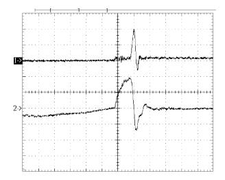
**Fig. 3.** Oscillograms of voltage pulses (1) on the anode of a laser head (vertical scale 65 kV/div) and current (2), running through the SOS-diode and shunt  $R_{\rm sh1}$  (vertical scale 620 A/div) under no-load conditions. The horizontal scale is 50 ns/div.
