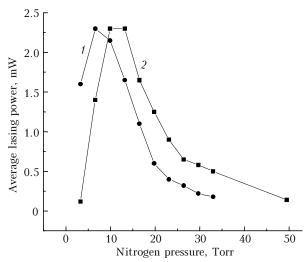
Fig. 5. Dependences of the average radiation power of the nitrogen laser pumped by longitudinal discharge on the active medium pressure for two Y-shaped cathodes of various length: d equal to 23 mm (1); to 100 mm (2). Pulse-periodic mode at the pulse repetition frequency of 10 Hz.
