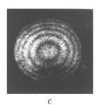
Fig. 8. The interference patterns localized in the plane of the diffuser image formation (a, b) and in the hologram plane (c), which characterize longitudinal motion of the diffuser when  $|R_1| = l_1$ .
