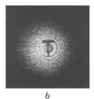
**Fig. 7.** The interference patterns localized in the plane of the diffuser image formation characterizing its longitudinal motion:  $R_1 = 350 \text{ mm}$  (a);  $R_1 = 125 \text{ mm}$  (b).
