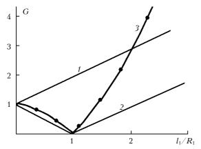
**Fig. 4.** Dependences of the interferometer sensitivity coefficients on the radius of curvature of a spherical wave front for  $l_1 = 250$  mm:  $G_1$  (1);  $G_2$  (2);  $G_3$  (3).
