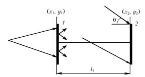
**Fig. 1.** Diagram of the Fresnel hologram recording: 1 is the matt screen; 2 is the photographic plate.
