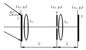
**Fig. 3.** Diagram of recording the interference pattern localized in the hologram plane: 2 is the hologram; 3 is the interferogram recording plane;  $L_1$  and  $L_2$  are the lenses; p is the spatial filter.
