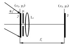
Fig. 2. Diagram of recording the interference pattern localized in a plane of the diffuser image formation: 2 is the hologram; 3 is the interferogram recording plane;  $L_1$  is the lens; p is the spatial filter.
