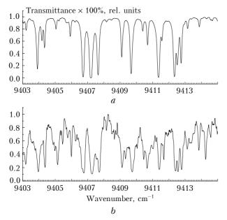
**Fig. 4.** Water vapor absorption spectrum in 9403-9415 cm<sup>-1</sup> region: calculated with the use of Ref. 9 (*a*) and obtained in this work (*b*).
