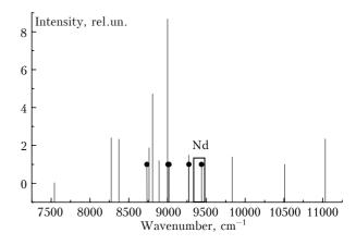
Fig. 3. Water vapor absorption bands in the range of Ndglass laser radiation.
