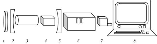
**Fig. 1.** Block-diagram of the experimental setup: interferometer (1), cavity mirrors (2 and 5), heated cell (3), active element (4), diffraction spectrograph DFS-8 (6), CCD photodetector (7), and PC (8).
