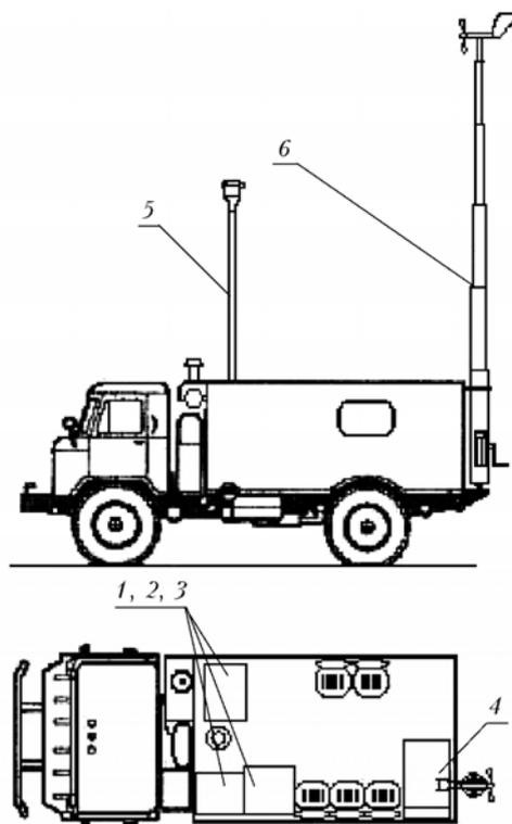
**Fig. 1.** The appearance of the AKV-2 station: posts with the measuring instrumentation (1, 2, and 3); power module (4); aerosol-gas intake (5); meteorological station based on the telescopic mast of KhZh4.115.025Sp type (6).
