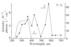
Fig. 1. Transmission spectrum (T) of the UFS glass filter used (1) and the spectrum of the net radiation passing through the front wall of the quartz reactor, measured with the interference filters (2).
