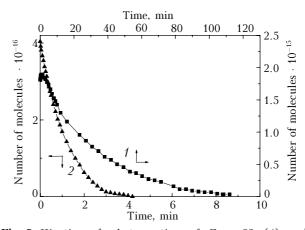
**Fig. 3.** Kinetics of photosorption of Freon 22 (1) and Freon 134a (2) on MgO. Temperature  $\sim 300$  K, Freon 22 initial pressure of 1 Pa, and that of Freon 134a of 2 Pa.
