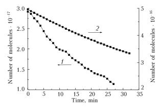
**Fig. 4.** Kinetics of photosorption of trichloroethane (1) on MgO surface and Freon 134a on CaCO<sub>3</sub> (II) (2). Temperature  $\sim 300$  K, trichloroethane initial pressure of 4.6 Pa, and that of Freon 134a of 1 Pa.
