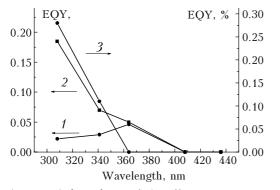
**Fig. 5.** Spectral dependence of the effective quantum yield (EQY) of photosorption of Freon 134a on  $CaCO_3$  (II): after the 30 min irradiation by the net radiation of the DRSh-250 mercury lamp in Freon 12 (1); after the additional 120 min irradiation by the net radiation in Freon 134a (2); photoadsorption of oxygen from the dried air (3).
