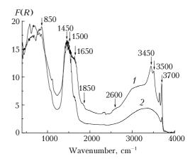
**Fig. 6.** Spectra of diffuse reflection in the IR spectral region for MgO after the photosorption of Freon 134a (1) and MgO heated at 620 K in vacuum (2).
