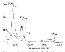
Fig. 2. Spectra of diffuse reflection in the IR region for initial MgO kept in air for a long time (1) and MgO heated in air at 773 K for 2 h (2).
