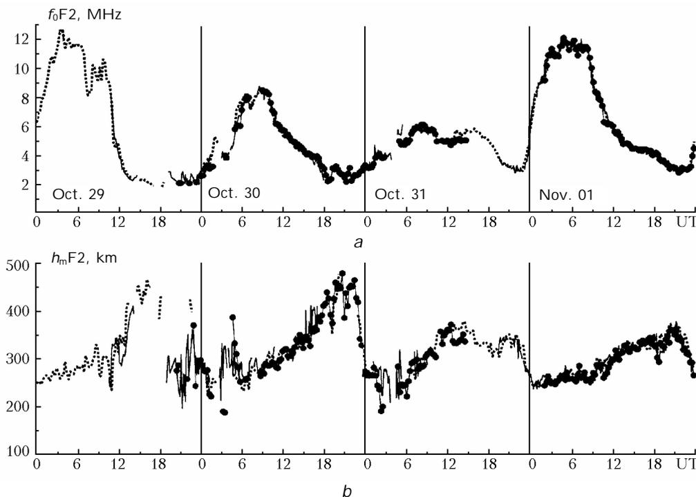
Fig. 3. Dynamics of the critical frequency  $f_0F2$  (a) and the altitude of the maximum  $h_mF2$  (b) during the magnetic storm on October 29–November 1, 2003: DPS-4 digisonde data (dashed line), FMCW sounder data (line with circles), and IS radar data (solid line).
