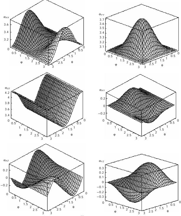
Fig. 2. Components of the polarizability tensor (in Å<sup>3</sup>) of N<sub>2</sub>...Ar complex at  $R = R_e$  and  $r = r_e$ ; the angles  $\theta$  and  $\phi$  are measured in radians.
