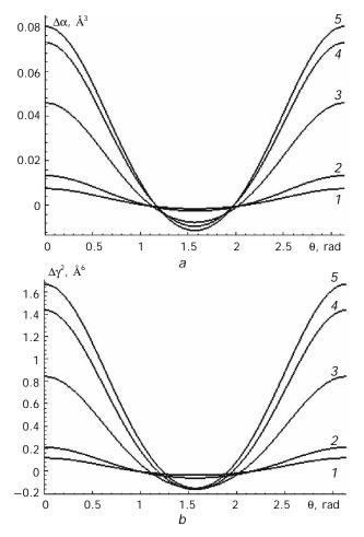
Fig. 3. Variation of the non-additive part of the mean polarizability (*a*) and the square polarizability anisotropy (*b*) of N<sub>2</sub>...Y complexes at  $R = R_e$  and  $r = r_e$ : N<sub>2</sub>...He (1), N<sub>2</sub>...Ne (2), N<sub>2</sub>...Ar (3), N<sub>2</sub>...Kr (4), N<sub>2</sub>...Xe (5).
