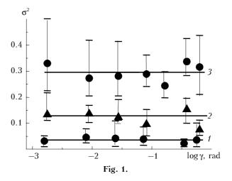
Since the receiver field of view in snowfalls is always larger than the diffraction angle, we found no effect of the receiver field of view on the measured variance in both of the beams. This effect is also absent in the case of no precipitation. The contribution of aerosol scattering in this case is low.
