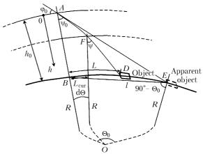
Fig. 1. Real and apparent locations of the surface object viewed from aboard an aircraft.
