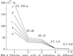
**Fig. 1.** Effective outer scale of turbulence for different vertical profiles of the outer scale (6). Plain surface,  $a_t = 0.5 \text{ m}$ ; *N* is the number of the model in Eq. (6);  $h_0 = 3$  (*a*), 6 (*b*), 12 (*c*), 24 (*d*), 48 m (*e*).
