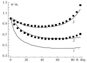
**Fig. 3.** Normalized root-mean-square deviation of the image jitter vs. the slope steepness of a single mountain.  $P_0 = 5$  km, z = 0.5 km,  $h_0 = 20$  m; n = 1 (1), 2 (2), 8 (3). Dots near the curves 2 and 3 show the equivalent dependences corresponding to the exponential profile n = 1 and calculated at z = 1.4 km (for profile 2, n = 2) and z = 4.6 km (for profile 3, n = 8).
