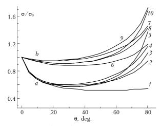
**Fig. 5.** Normalized rms deviation of image jitter for the system of two mountains;  $h_0 = 20$  m, groups *a* and *b* correspond to different versions of the mountain, at which the telescope is installed: (*a*) mountain with highly steep slopes:  $P_0 = 3$  km,  $z_0 = 0.3$  km; (*b*) mountain with moderately steep slopes:  $P_0 = 3$  km,  $z_0 = 3$  km.
