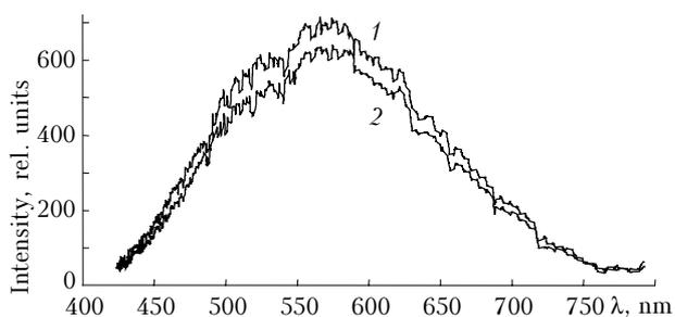
**Fig. 1.** The spectra of solar radiation before (1) and after (2) transmission through the film with the 0.1% m/m PE luminophore content. The spectra are not corrected for the spectral sensitivity of the photodetector used.
