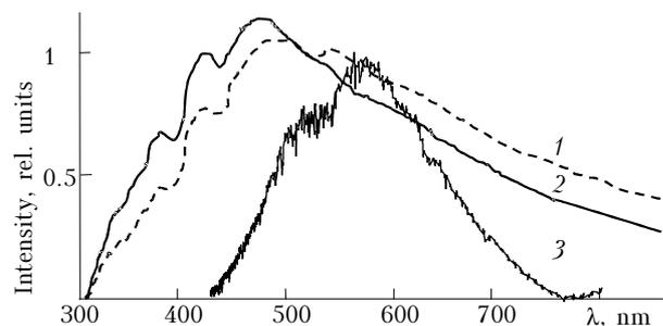
**Fig. 3.** Energy distribution in the solar spectrum: net (1) and diffuse (2) radiation (clear sky); the spectrum recorded with the Kwarts-3102V spectrometer (3).
