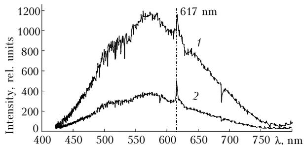
**Fig. 2.** The spectra of solar radiation transmitted through the HPPE film with 5% m/m addition of PLE luminophore (1) and transmitted by the HPPE film with 3% m/m addition of PLE luminophore (2). The spectra are not corrected for the spectral sensitivity of the photodetector used.
